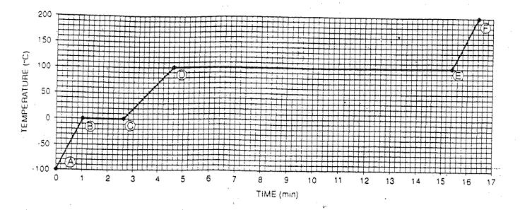
note: energy is being added to 50 grams of water at a constant rate, the graph shows the temperatures recorded when a sample of water was heated for almost 17 minutes.
